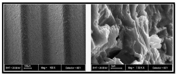
Scanning electron micrographs of a TiO blasted surface
