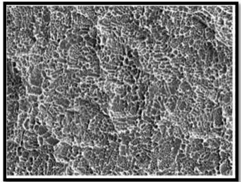
Scanning electron micrograph of an implant surface processed with dual acid-etching procedure
