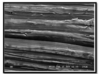
Scanning Electron Micrograph of Turned or Machined Dental Implant Surface
