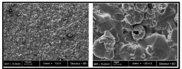
Scanning electron micrographs of a plasma-sprayed hydroxyapatite coating surface
