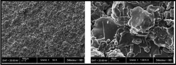
Scanning electron micrographs of a Titanium plasma sprayed surface
