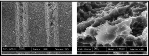
Scanning electron micrographs of an SLA surface on Titanium dental implant
