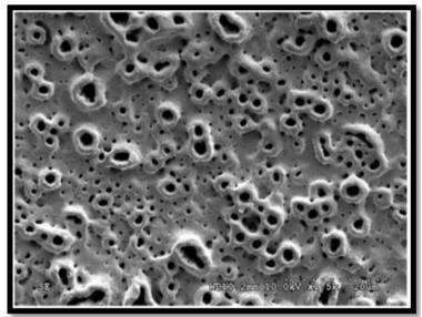
Scanning Electron Micrograph of Anodic Oxidation
